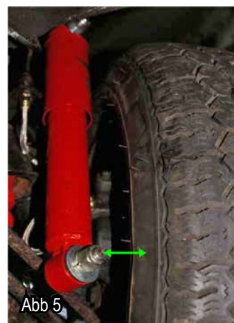
Abb 5 Mindestabstand 12 mm Jeu minimum 12 mm Minimum clearance 12mm
