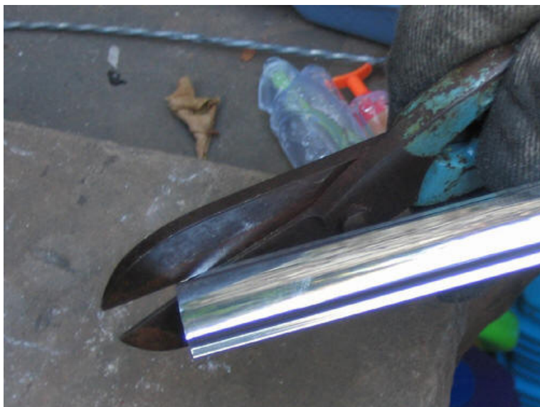
For each piece of chrome strip, chamfer the end lips with some tin snips (not necessary for the corner pieces)
