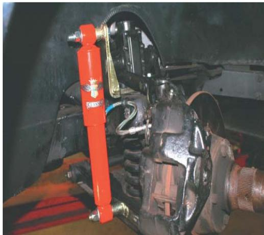
MGA with disc brake Brake hos on top
