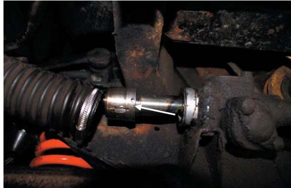
Remove the lock nut and unscrew the track rod
