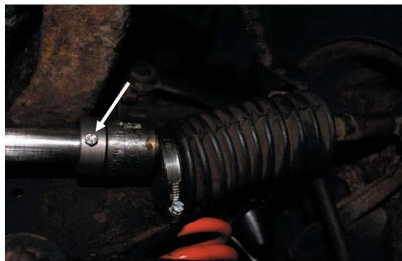
lockscrew keeps steering lock in position
