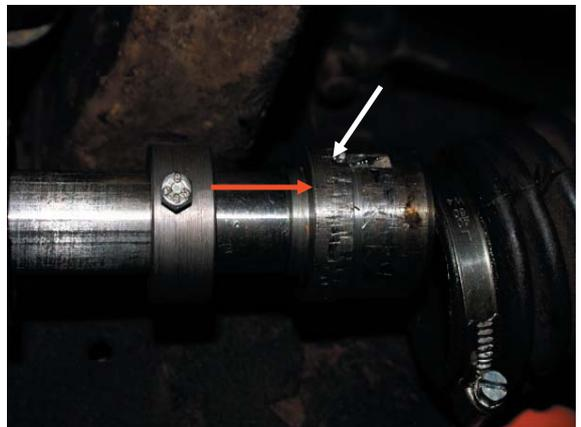
Push the steering lock in outer position
