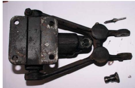
**The telescopic dampers are installed on the rear of the suspension with the upper mounting plate (VA80 MGB-1LH / VA80MGB-1RH ) fitted below the lever arm unit.**
